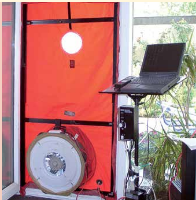
Fan for an air pressure test
