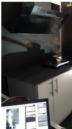
The experimental setup for vapour collection in the kitchen studio. Picture: PHI
