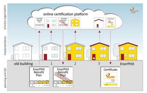
First the entrance door and windows, then facade and roof: The EnerPHit Retrofit Plan allows forward-thinking planning of retrofit steps and facilitates achievement of the EnerPhit Standard.
